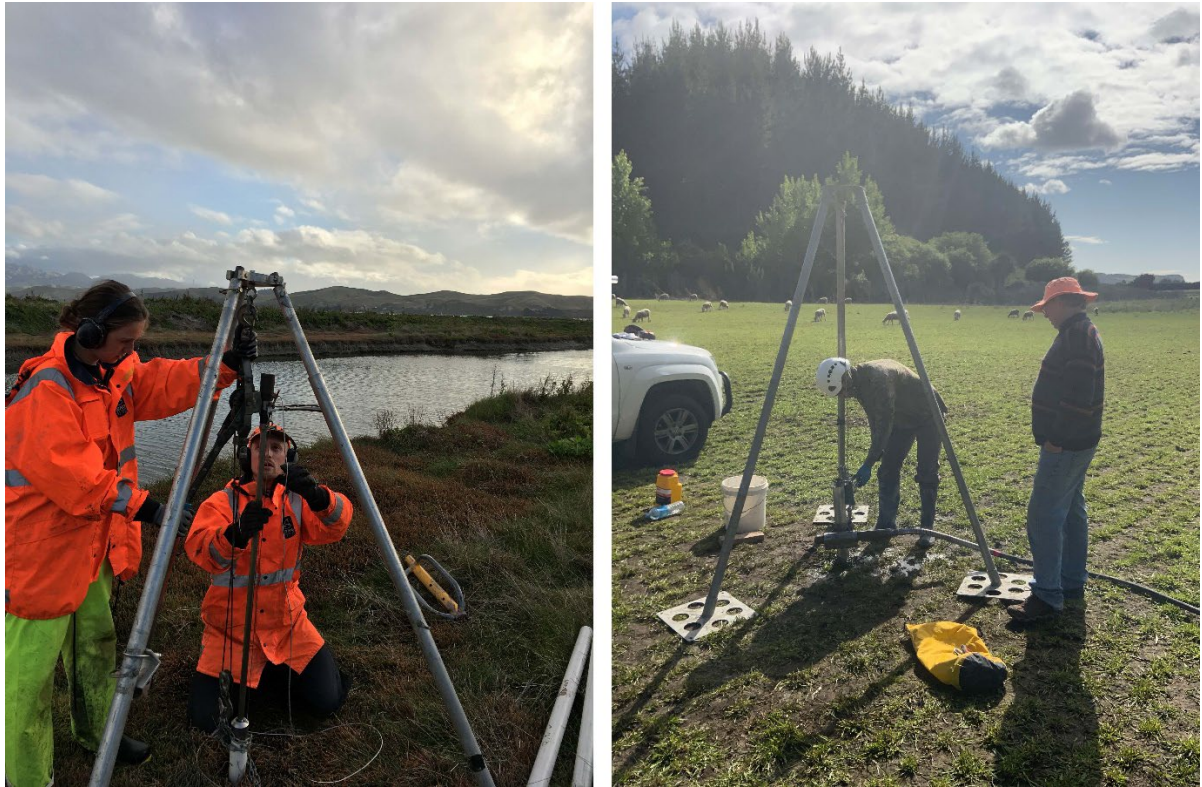
Figure 7. LEFT: Piston corer in use. RIGHT: Vibrocorer in use. Photographs provided by Dr. Kate Clark (GNS Science).
